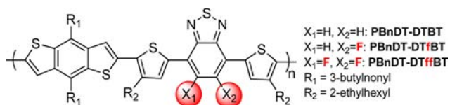
Figure 1. The structures of PBnDT-DTBT (“0F”), -DTfBT (“1F”) and -DTffBT (“2F”).
